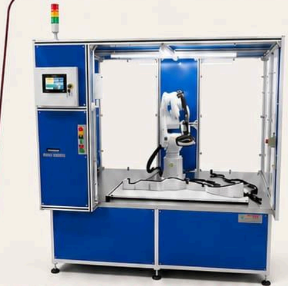
• ROBOTIC VISION INSPECTION MACHINE •
